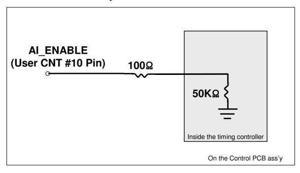
Fig. The AI\_ENABLE Circuit Block Diagram
