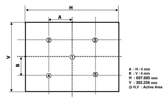
FIG. 2 The Position of Points for Luminance Measure
