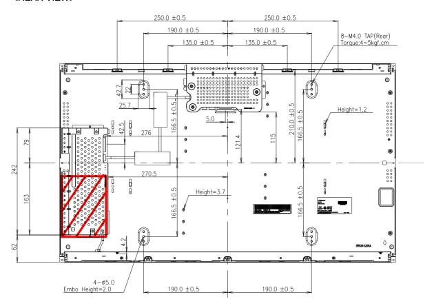
NOTES 1.JUNSPECIFIED TOLERANCES TO BE  $\pm 0.5$ MM 2.TILT AND PARTIAL DISPOSITION TOLERANCE OF DISPLAY AREA ARE AS FOLLOWING. (1) Y-DIRECTION: I A-B I  $\leq$  1.5 (2) X-DIRECTION: I C-D I  $\leq$  1.5
