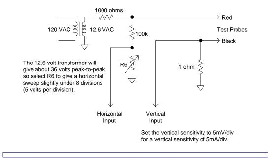
Here is a simple version with a single voltage range of about 18 volts peak and a current limit of about 18 milliamps peak. The transformer is an ordinary "filament" transformer or similar with a single secondary. This one-range tracer is quite useful for quick checking of zeners, transistor junctions, LEDs, and most other semiconductors.
