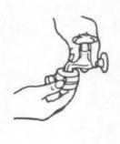
Connect the inlet hose to the water tap adapter by pulling down the collar of the hose end.
