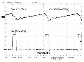
Figure 13. VOLTAGE RIPPLE AT INPUT (I<sub>0</sub> = 3 A)
