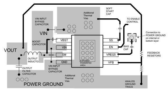
Figure 16. PCB Layout
