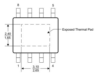
Figure 15. Thermal Pad Dimensions
