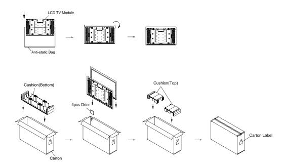
Figure.9-1 packing method
