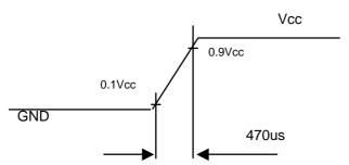
Note (3) The specified power supply current is under the conditions at Vcc = 12V, Ta = 25  $\pm$  2  $^{\circ}$ C, f<sub>v</sub> = 60 Hz, whereas a power dissipation check pattern below is displayed.
