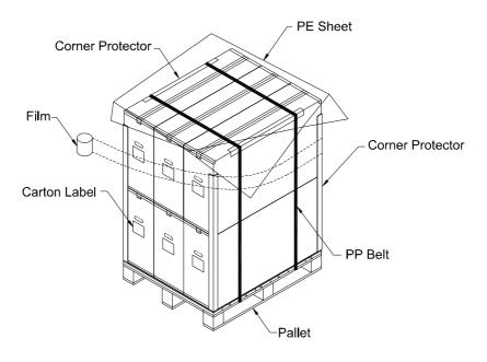
Figure.9-2 packing method
