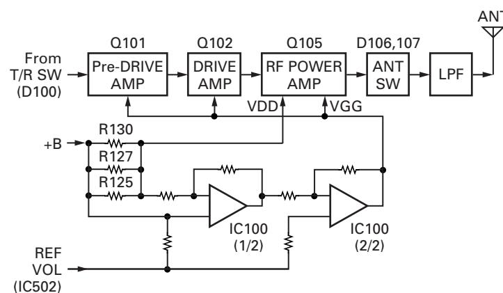
**Fig. 8 Drive and final amplifier and APC circuit**
