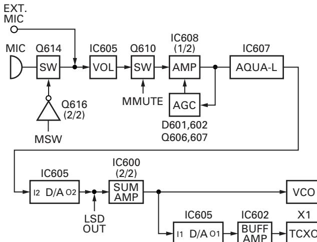
**Fig. 7 Microphone amplifier**
