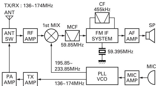
**Fig. 1 Frequency configuration**
