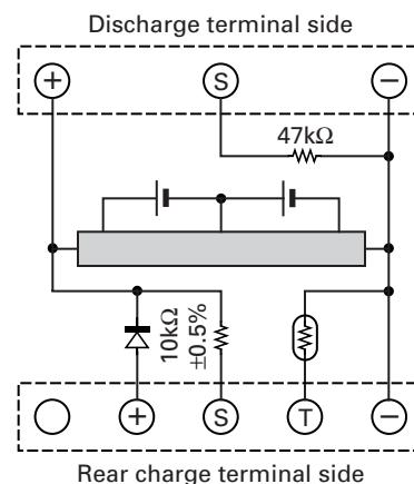
■ KNB-32N Internal wiring
