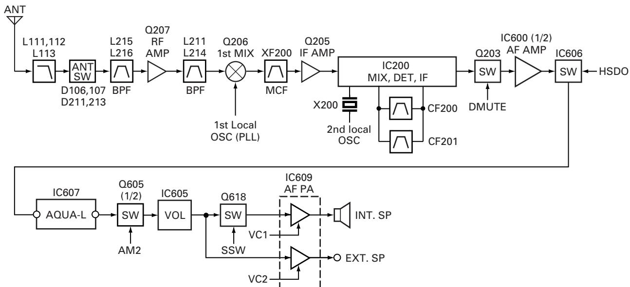
**Fig. 2 Receiver section**
