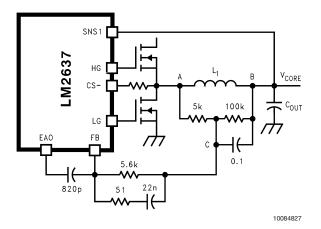
FIGURE 9. Dynamic Voltage Positioning by Utilizing
