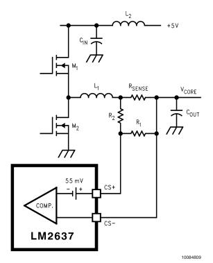
FIGURE 5. Current Limit via Current Sense Resistor
