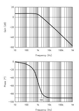
FIGURE 7. Control-to-Output Bode Plots
