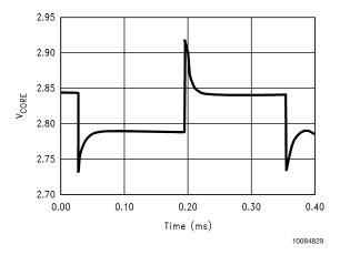
FIGURE 11. Load Transient Response with DVP: 0A to 14A, ESR = 9.4 m $\Omega$ , Droop Resistor = 4 m $\Omega$
