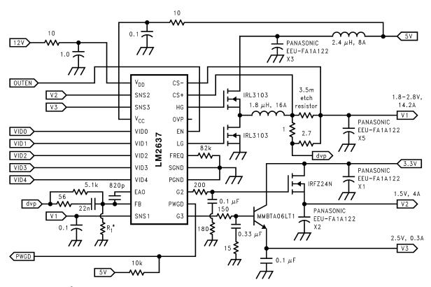
$^{*}$  R $_{\parallel}$  is for raising the switcher output voltage slightly. Its value depends on the output voltage.
