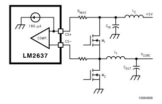
FIGURE 4. Current Limit via High-Side FET V<sub>DS</sub> Sensing
