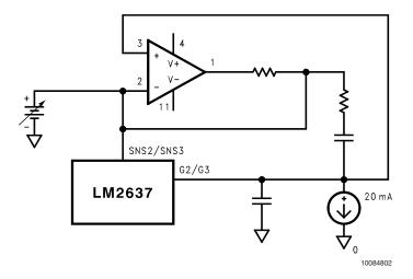
FIGURE 1. LDO Controller Test Circuit
