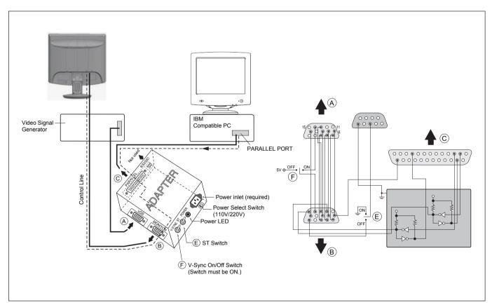
Figure 1. Cable Connection
