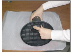
Push the two latches on the bottom to the inside. (Reference the #1-2)
