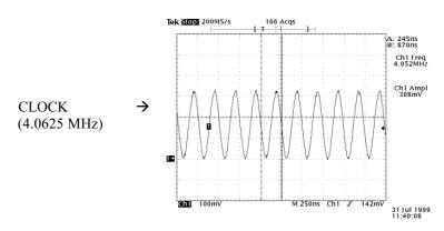
Location of Measurement: See schematic diagram Page03/Y1/Pins1,2
