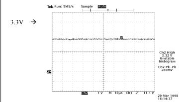
Location of Measurement: See schematic diagram Page03/ All power supply of U4
