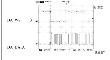
Location of Measurement: See schematic diagram page13/ U19,Pin2
