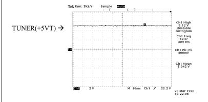
Location of Measurement: See Schematic Diagram Page02/U1, Pin8
