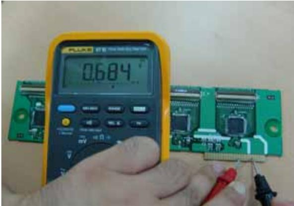
Normal diode value. (in case of TI IC =0.6 ~ 0.7)
