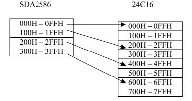
E.g. , if data is located at address 100H in SDA2586, it must be at 200H in 24C16. The first 256 addresses from 0 to FF are the same for both ICs.
