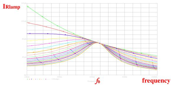
Figure 2. Lamp Current Vs Frequency, Rlamp
