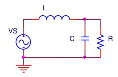
Figure 3. Simplied RCL tank circuit
