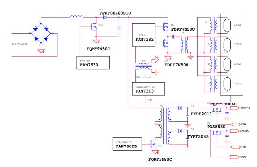
Figure 5.Super IP Fairchild Block Diagram
