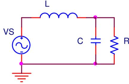
Figure 3. Simplified RCL tank circuit
