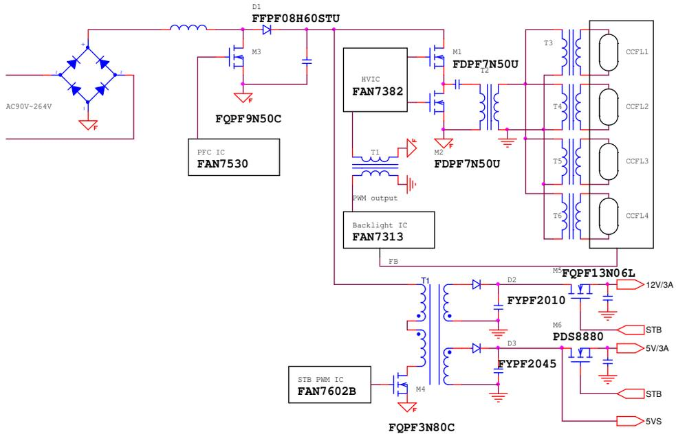
Figure 5. Super IP Fairchild Block Diagram
