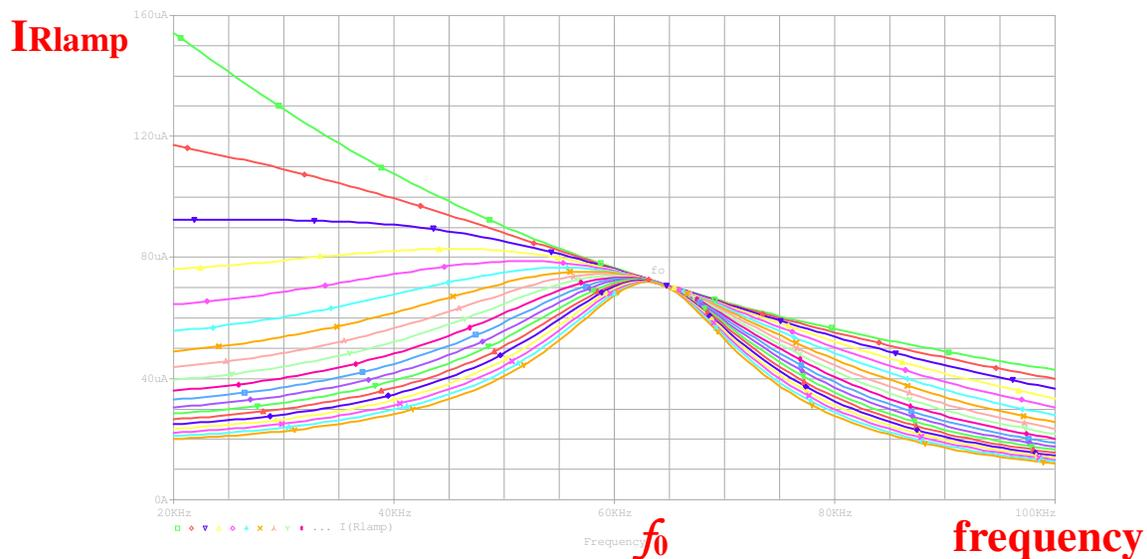
Figure 2. Lamp Current Vs Frequency,  $R_{lamp}$
