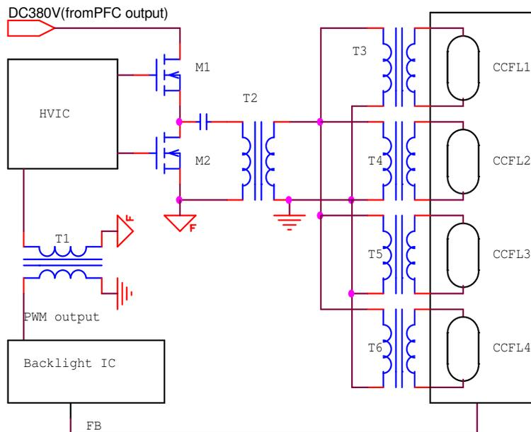
Figure 1. Super IP LCD TV Power Block
