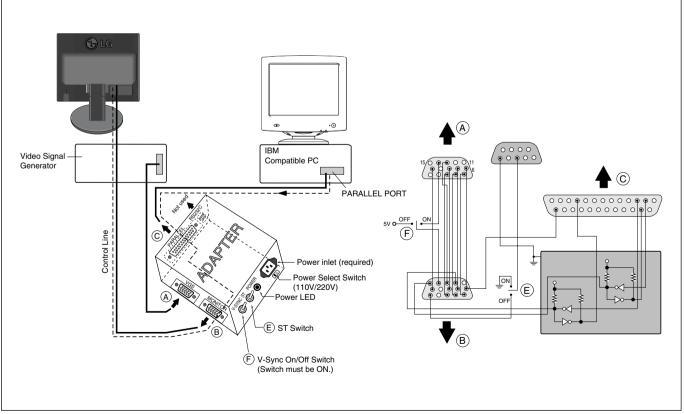
Figure 1. Cable Connection
