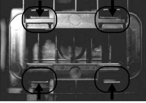
After finished repair, necessarily push 4ea Latches to inside for restoration.
