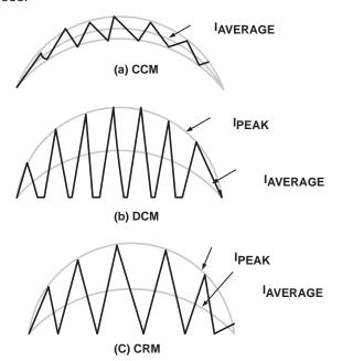
**Figure 2. PFC Inductor Current Profiles**
