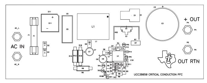
Figure 5. Reference Design Board Layout
