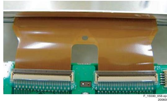
Figure 9-10 Flexible Printed Circuit
