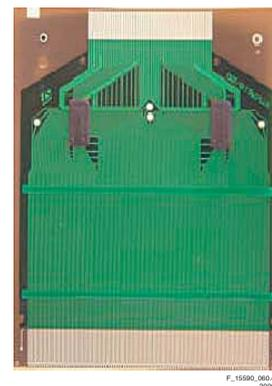
Figure 9-12 Tape Carrier Package
