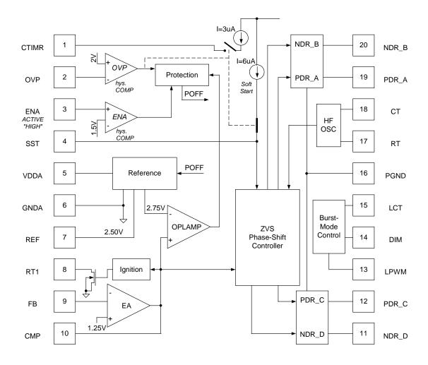
Figure 2. Functional Block Diagram
