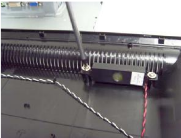
7. Loose and remove 2 Screws and pull out Speaker Cable
