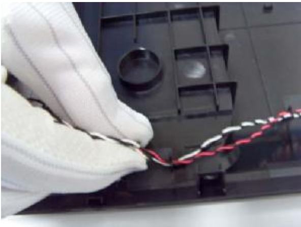
7. Loose and remove 2 Screws and pull out Speaker Cable
