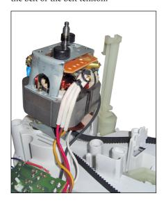
Remove the Belt tension, by lifting it a little bit (green arrow) and pulling it in direction of the red arrow.
