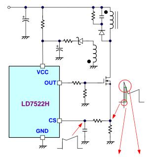
R-C filter is needed whenever the negative spike is exceed -0.3V or the total spike width is over 350nS LEB period.
