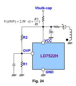
As similar behavior like OLP, whenever the voltage on the OVP pin is higher than the threshold voltage 2.5V, the output gate drive circuit will be shutdown simultaneous thus to latch off the switching of the power MOSFET. Whenever
