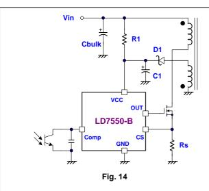
A 350nS leading-edge blanking time is included in the input of CS pin to prevent the false-trigger caused by the current spike and further to eliminate the need of R-C filter which is usually needed in the typical UC384X application (Fig. 15).
