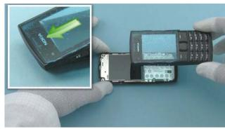
8) Release the top end of the A-COVER by lifting up the bottom end and pushing to the direction shown. The A-COVER and the KEYMAT can now be separated.
