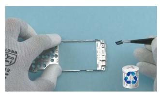
23) Remove the EARPIECE adhesive with tweezers. Do 24) Peel off one corner of the DOMESHEET with the not use it again. Discard it.
