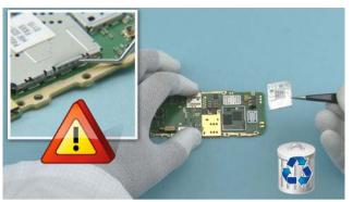
26) Use the dental tool to lever out the BB SHIELDING LID. Be careful not to damage the components nearby! Discard the BB SHIELDING LID.
