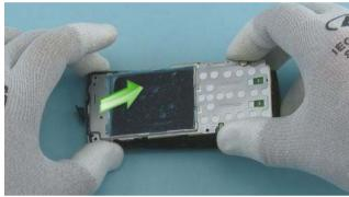
15) Carefully pull the ENGINE BOARD to the direction shown.
