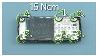
1) Tighten the six Torx+ size 6 screws to the torque of 15 Ncm in the order shown.
