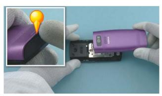
4) Use the BATTERY COVER release notch to open the BATTERY COVER. Remove the BATTERY COVER.
