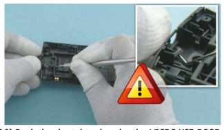
36) Push the dental tool under the MICRO USB DOOR as shown and lift it up gently. The clip holding the MICRO USB DOOR is released. Be careful not to damage the MICRO USB DOOR or the D-COVER with the sharp end of the dental tool!
