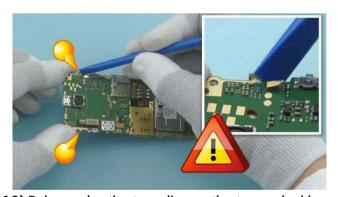
18) Release also the two clips on the top end with the SS-93. Be careful not to damage the nearby components!
