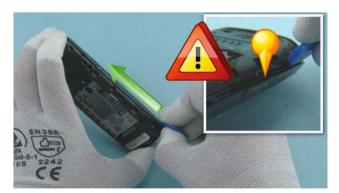
6) Slide the SRT-6 to the direction shown to release the left side of the A-COVER. Be careful not to damage the MICRO SD CARD DOOR or the MUSIC KEY!
