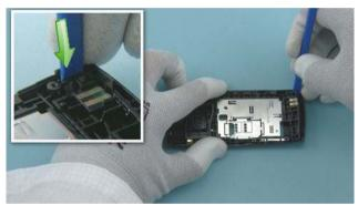
34) Push the SS-93 to the shown place to release the GSM ANTENNA.
