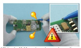
17) Use the SS-93 to release the two shown clips holding the UI SHIELD. Be careful not to damage the nearby components!
