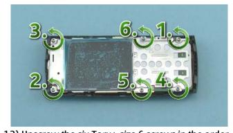
12) Unscrew the six Torx+ size 6 screws in the order shown.
