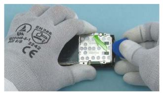
14) Use the SRT-6 to lift up the ENGINE BOARD.
