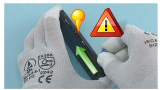
7) Slide the SRT-6 to the direction shown to release the right side of the A-COVER. Be careful not to damage the SIM2 CARD DOOR or the VOLUME KEYS!
