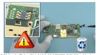
28) Peel off the SIM CARD PROTECTIVE TAPE with the dental tool. Be careful not to damage the components nearby! Remove the SIM CARD PROTECTIVE TAPE with tweezers. Discard it.
