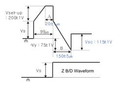
(Fig. 2) Y, Z set-up Waveform
