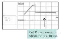
(Fig. 3) When the Set\_Down FET is damaged
