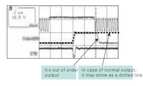
(Fig. 7) When IC output of COF is poor
