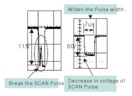
(Fig. 6) When SCAN IC output is short
