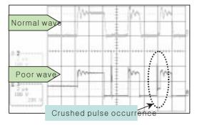
(Fig. 1) When the ER\_FET is damaged
