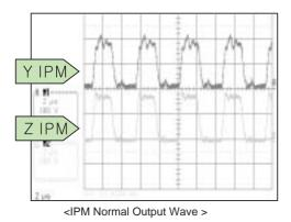
Measurance position: Sustain section enlarge the after measuring B103 wave of Y B/D and B37 wave of Z B/D. (Full White Pattern)
