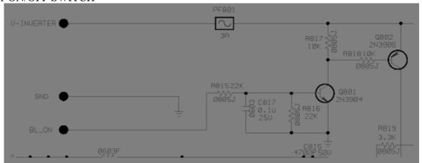
The turn-on voltage was controlled by R815 and R816. The inverter was turned on or off by the switching transistors Q801 and Q802.
