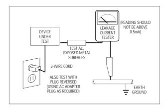
Fig. 1-1 AC Leakage Test
