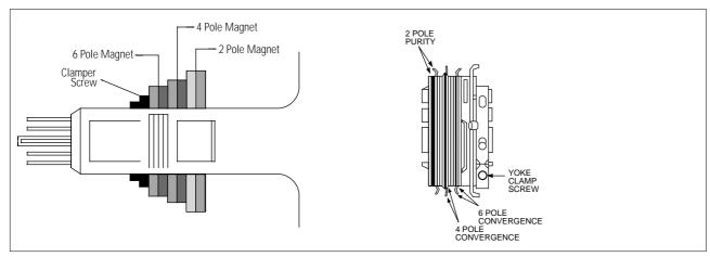
Fig. 4-2 Convergence Magnet Assembly
