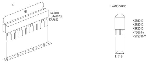
Fig. 2-1 Semiconductor Base Diagrams
