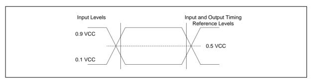
Figure 27. AC Measurement I/O Waveform
