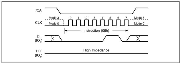
Figure 4. Write Enable Instruction Sequence Diagram
