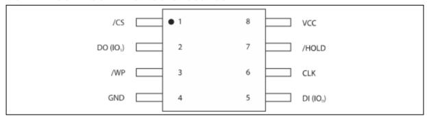
Figure 1a. W25X20CV Pin Assignments, 8-pin SOIC 150 / 208-mil (Package Code SN, SS)
