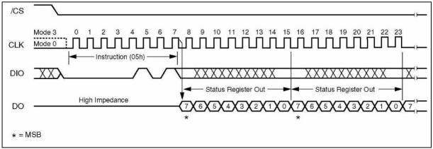
Figure 7. Read Status Register Instruction Sequence Diagram
