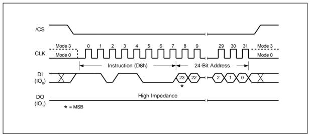
Figure 17. Block Erase Instruction Sequence Diagram
