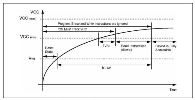
Figure 26a. Power-up Timing and Voltage Levels
