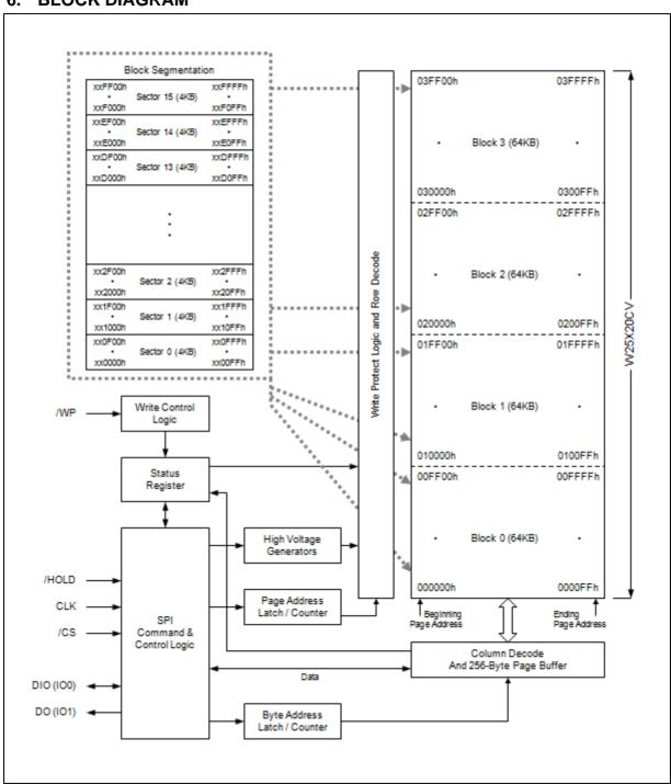
Figure 2. W25X20CV Serial Flash Memory Block Diagram
