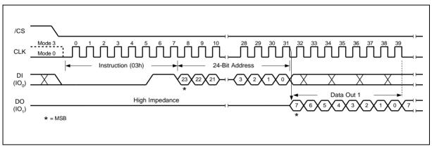
Figure 9. Read Data Instruction Sequence Diagram
