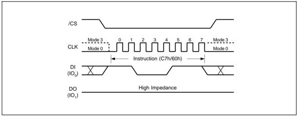
Figure 18. Chip Erase Instruction Sequence Diagram
