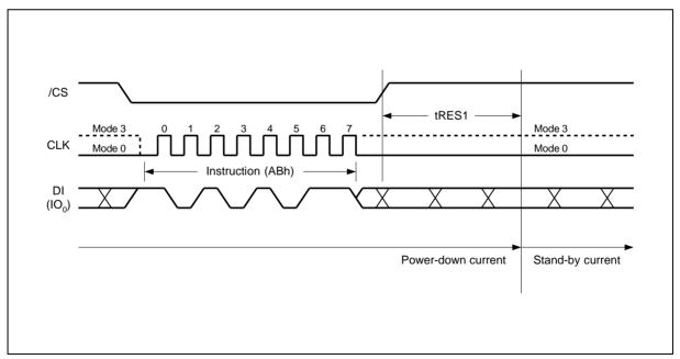
Figure 20. Release Power-down Instruction Sequence
