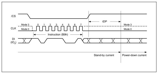
Figure 19. Deep Power-down Instruction Sequence Diagram
