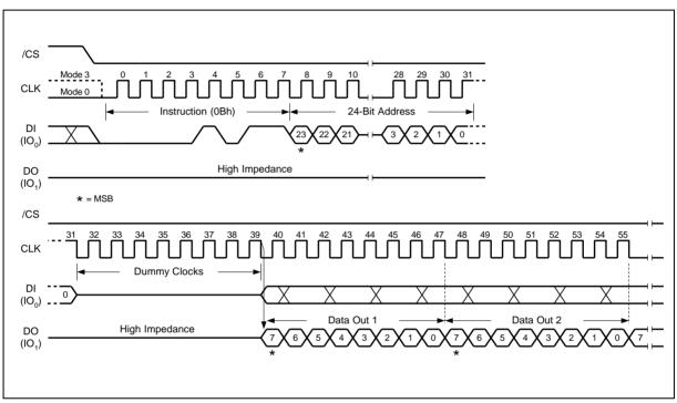
Figure 10. Fast Read Instruction Sequence Diagram
