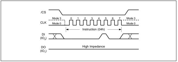
Figure 6. Write Disable Instruction Sequence Diagram
