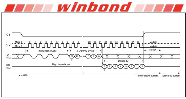
Figure 21. Release Power-down / Device ID Instruction Sequence Diagram
