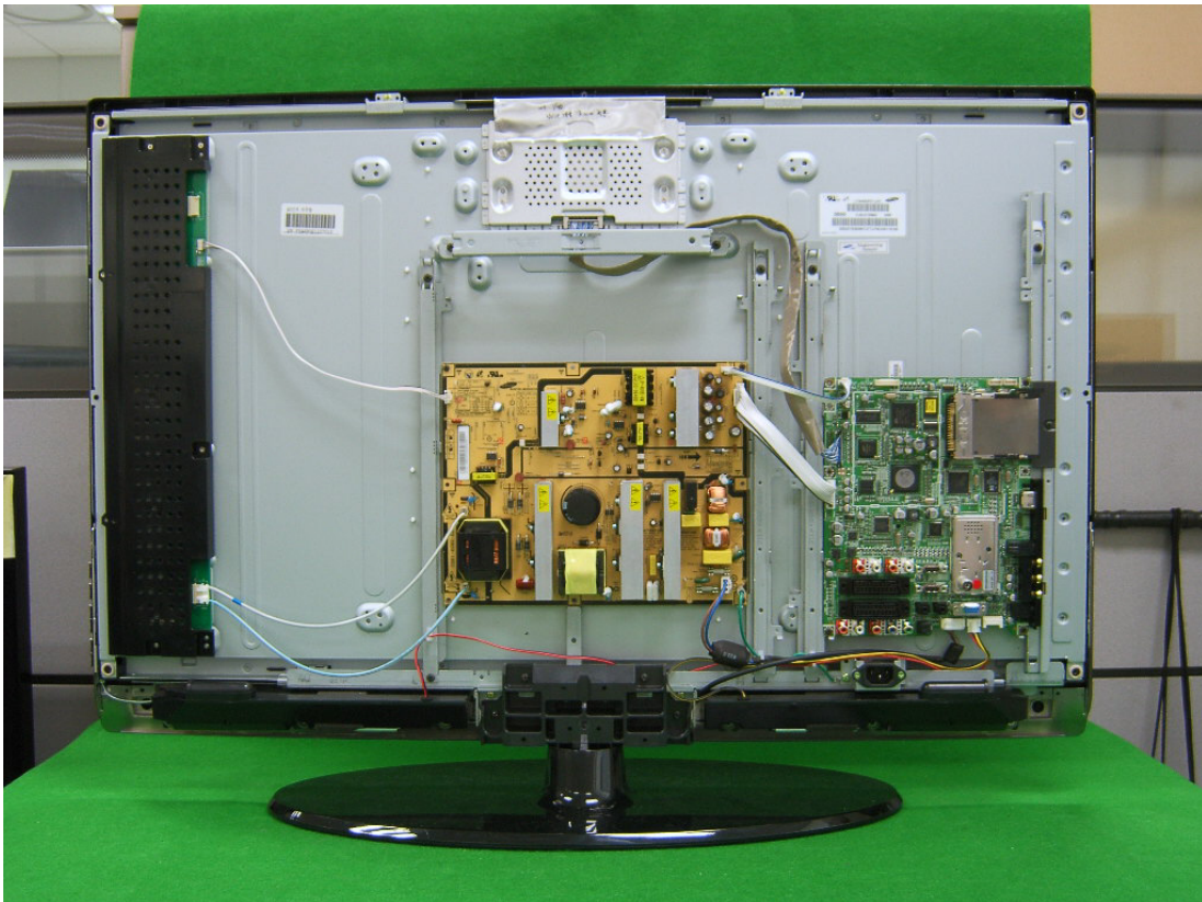
<Photo 4 > TU40EO – Internal View with IP-231135A
