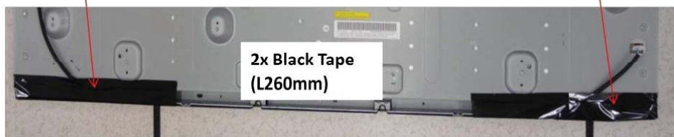
Figure 4-10 Light leakage solution (only for 37" model)
