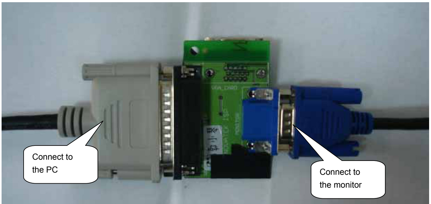
Figure 1 Cable Connection for Micom uploading
