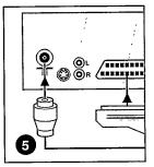
or, A device with a Euroconnector can be connected to the Euroconnector socket located at the back of the TV (a support bracket is provided for the Euroconnector cable on the back of the TV).
