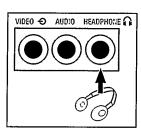
To connect headphones (The headphones used must be 8 to 1000 ohm, and 6.3 mm in diameter.)
