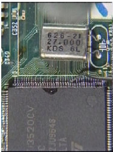
8. Most technicians forget to inspect for bridges after installing the IC. When power is turned ON, a bridge will take out the new IC or damage another related parts. Therefore it is important to inspect the pins for bridges before approving your own work.
