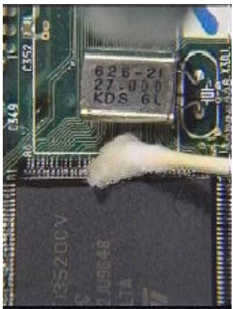
10. Remove the excess flux by spraying the area lightly with flux remover.
