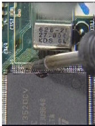
4. Check the IC position and solder another lead to hold the IC in place.
