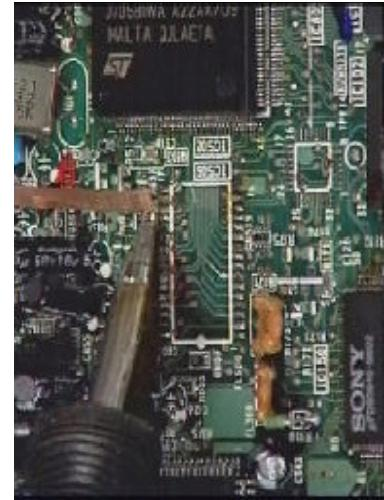
To solder all the IC leads without creating bridges, you need a constant tip temperature soldering iron.
