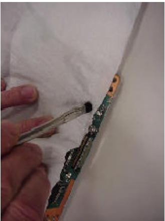
9. Using a low flux solder means you do not have to clean the board of flux with a flux remover....
