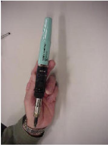
Put safety goggles on before using the butane torch. Circle the IC leads with the torch flame and flip the IC over when the IC is loose.
