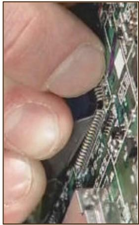
1. You must place the new blade at the legs where they meet the IC body. Angle the blade into the body slightly to avoid slipping off the IC legs.
