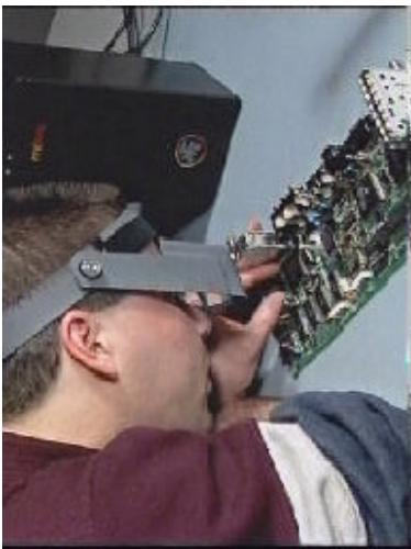
7. After soldering all the pins, run a dental pick across the pins to see if movement reveals an unsoldered one.
