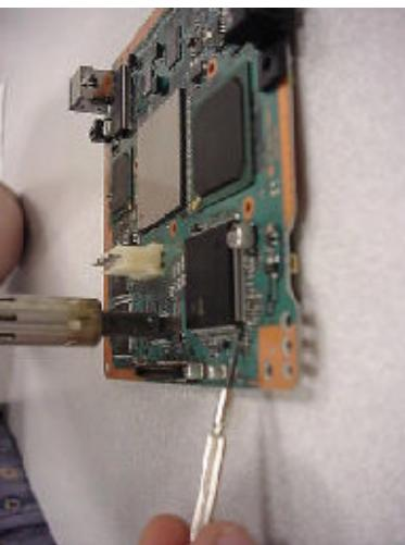
1. Apply the Chip Quick flux to all the leads of the IC. (Medium size IC shown for removal).
