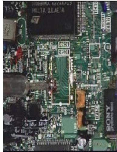
5. The remaining Chip Quick is removed with a solder wick. Move the wick in the same direction as the lands of foil.
