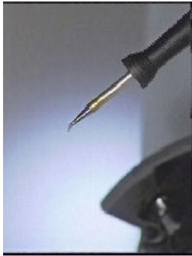
1. Whichever iron you use, clean the tip by dipping it into a cleaner or tinner. Kester and Multicore manufacture these. A dirty tip will cause you to mis-solder some IC leads as you drag the solder across the IC pins.
