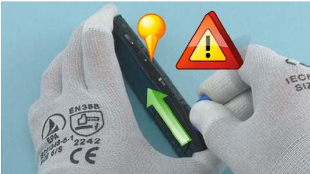
7) Slide the SRT-6 to the direction shown to release the right side of the A-COVER. Be careful not to damage the SIM2 CARD DOOR or the VOLUME KEYS!
