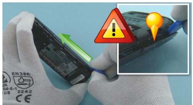
6) Slide the SRT-6 to the direction shown to release the left side of the A-COVER. Be careful not to damage the MICRO SD CARD DOOR or the MUSIC KEY!
