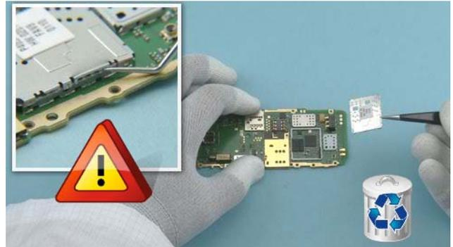
26) Use the dental tool to lever out the BB SHIELDING LID. Be careful not to damage the components nearby! Discard the BB SHIELDING LID.
