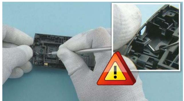
36) Push the dental tool under the MICRO USB DOOR as shown and lift it up gently. The clip holding the MICRO USB DOOR is released. Be careful not to damage the MICRO USB DOOR or the D-COVER with the sharp end of the dental tool!
