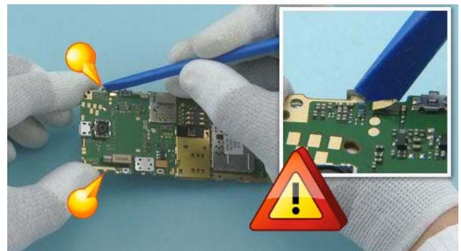
18) Release also the two clips on the top end with the SS-93. Be careful not to damage the nearby components!
