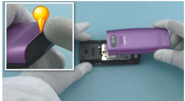
4) Use the BATTERY COVER release notch to open the BATTERY COVER. Remove the BATTERY COVER.
