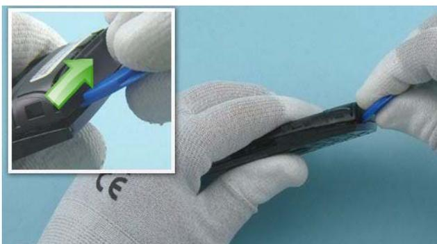
5) Insert the SRT-6 between the A-COVER and the D-COVER on the bottom end of the device. Slide the SRT-6 to the direction shown to release the bottom end of the A-COVER.
