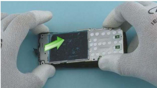
15) Carefully pull the ENGINE BOARD to the direction shown.
