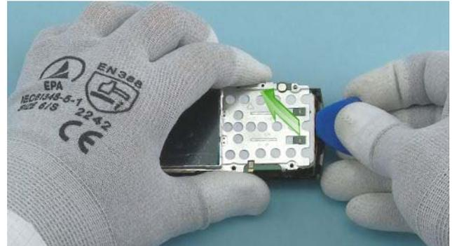
14) Use the SRT-6 to lift up the ENGINE BOARD.
