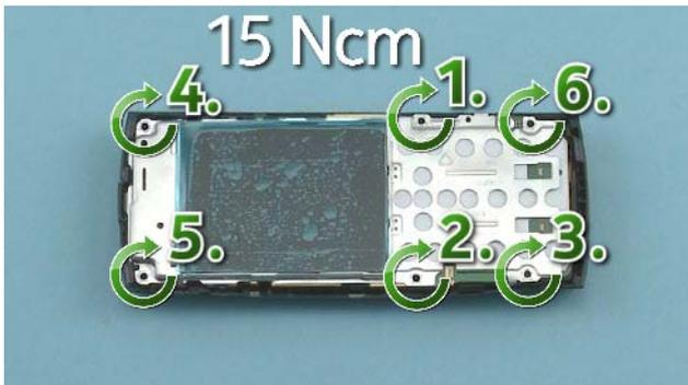
1) Tighten the six Torx+ size 6 screws to the torque of 15 Ncm in the order shown.
