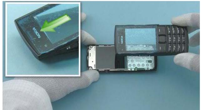
8) Release the top end of the A-COVER by lifting up the bottom end and pushing to the direction shown. The A-COVER and the KEYMAT can now be separated.
