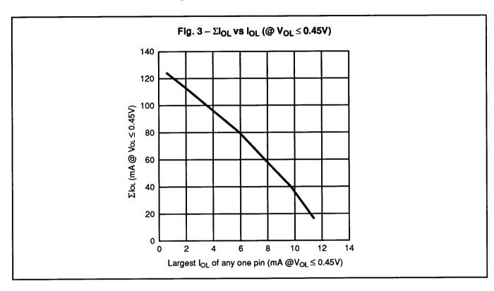
For instance, if one of the I/O lines has to sink 9mA, the total  $I_{OL}$  ( $\Sigma I_{OL}$ ) of all lines can be up to 45mA.
