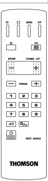
**Batteries:** Remove the lid at the back of the remote control and insert two 1,5 V batteries, TYPE LRO3 (AAA) or equivalent.
