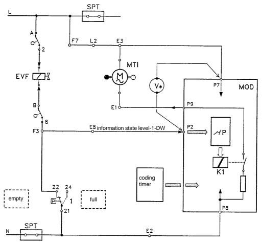
\* N1 in position "empty"  $\Rightarrow$  P2 in state "1" (220 V between P7 and P2) N1 in position "full"  $\Rightarrow$  P2 in state "0" (0 V between P7 and P2)
