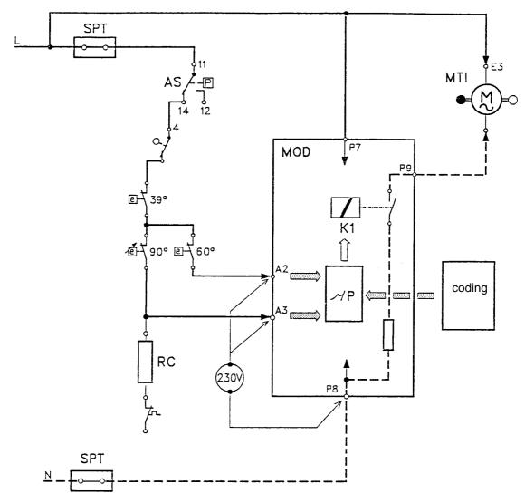
$\Rightarrow$  Input A2 in state "1" (220/230 V between clamps A2 and P8)  $\Rightarrow$  Input A3 in state "1" (220/230 V between clamps A3 and P8)
