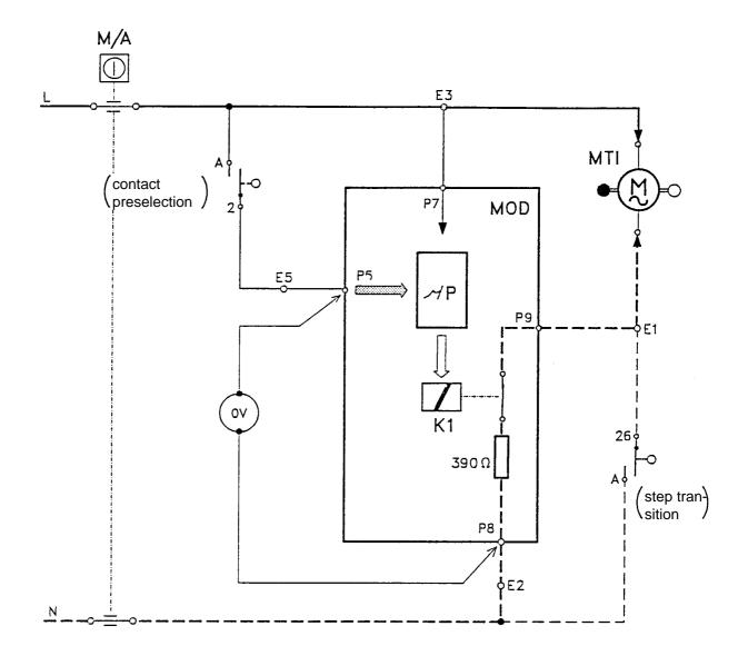
The entry of a washing program causes the opening of contact 2-A.
