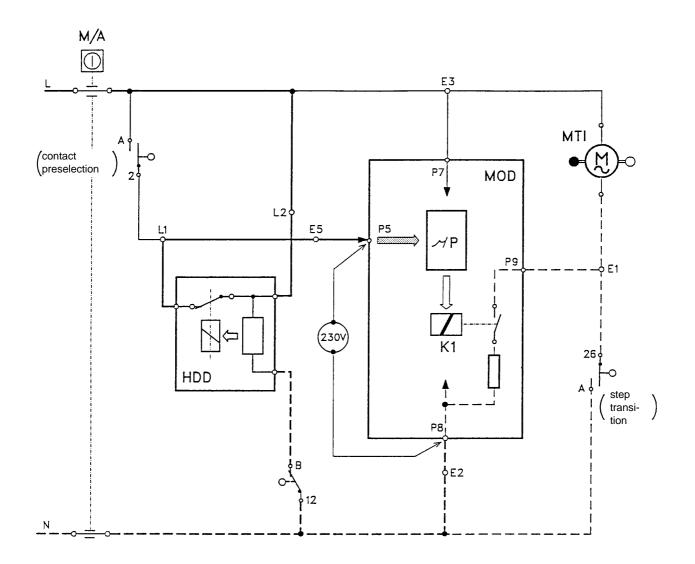
The selection of a start time delay entails the closing of the relay contact of the time link. This results in the transition from input P5 of the electronic system to state "1" (220/230V between P5 and P8).
