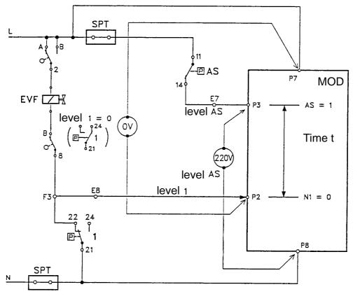
Input P2 changes from state "1" to state "0" (0 V between P7 and P2)  $\Rightarrow$  Selection of MTI; continuation of the PGS up to step 13.
