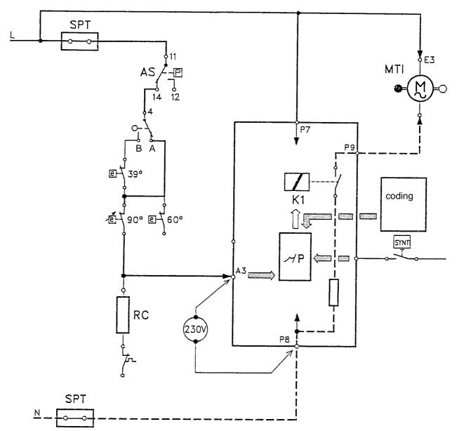
The **nonpressed** button for synthetics activates the thermostop function only by:
