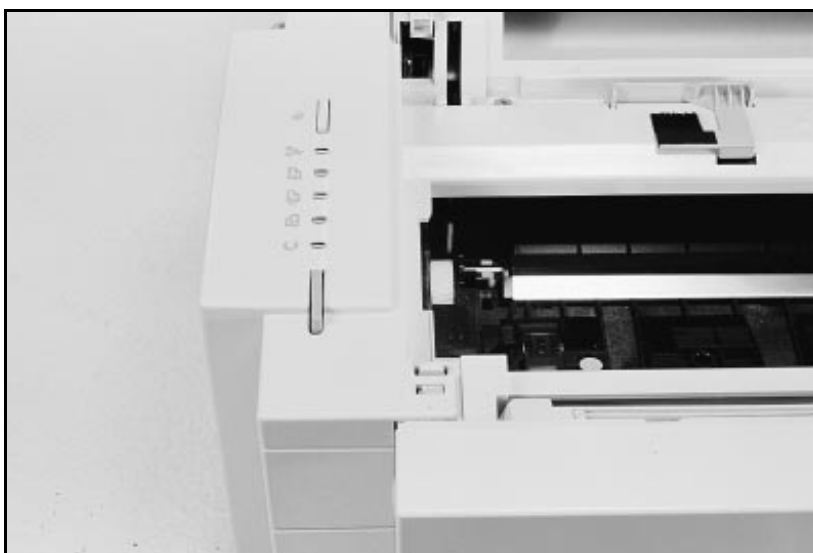
Figure 17 Left Side Cover Release Latch (5P/5MP shown)
