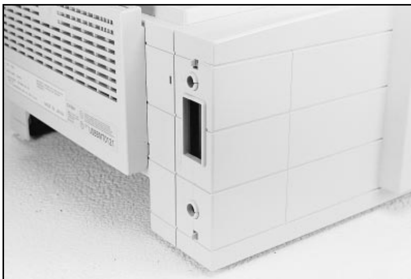
Figure 15 5P/5MP I/O Cover Release Tabs
