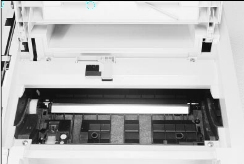
Figure 18 Removing the Top Cover Screws
