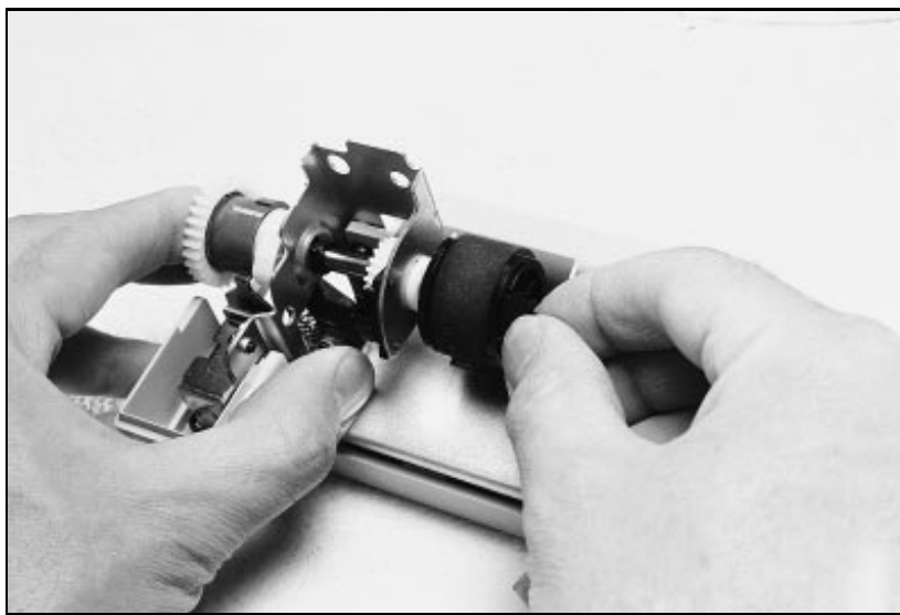
Figure 23 Replacing the Pickup Roller
