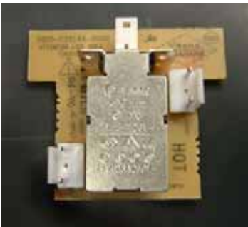
MAIN POWER SWITCH CONTROL
