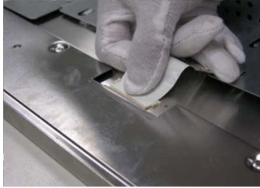
Pull out the LVDS cable
