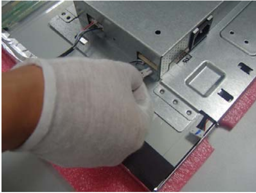
Pull out the lamp wire.
