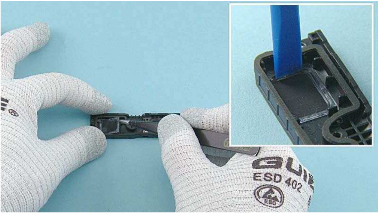
Place the IHF SPEAKER GASKET. Press it gently to activate the adhesive.
