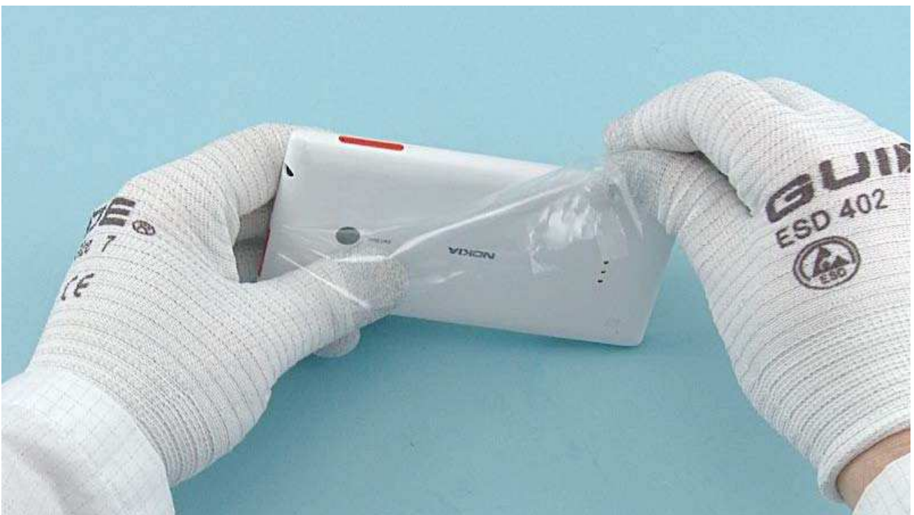
Remove the UNIBODY ASSEMBLY protective film.
