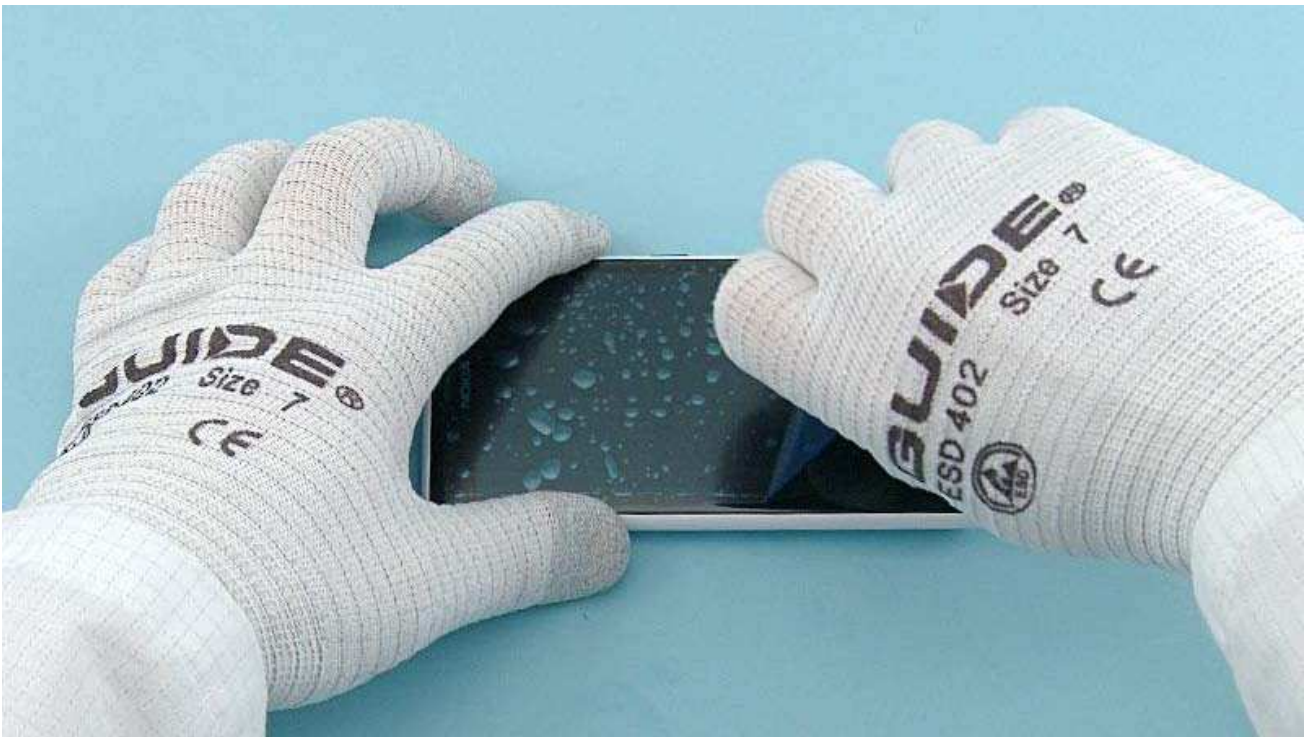
Remove the DISPLAY protective film.
