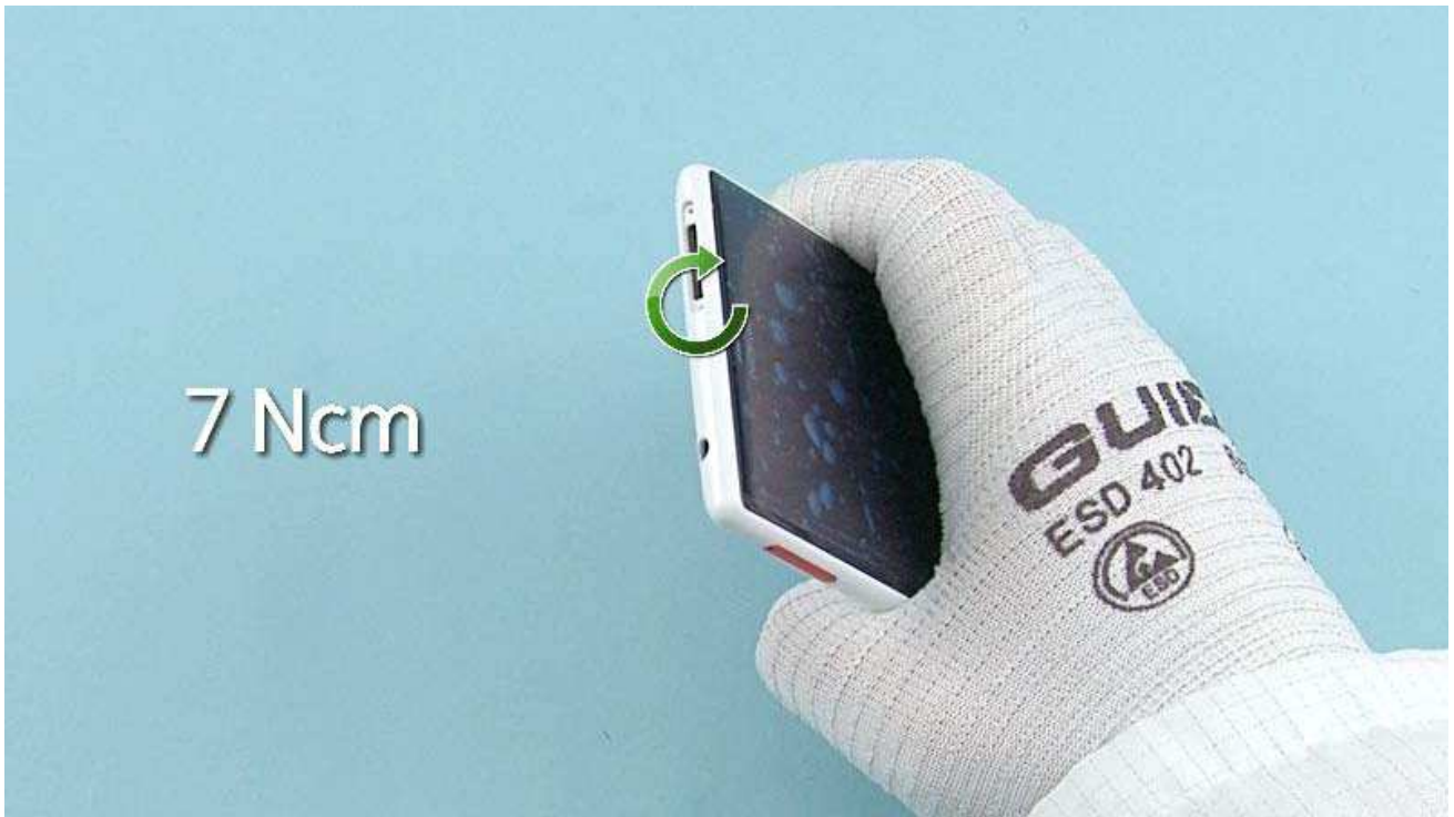
Fasten the TORX+ size 2 screw to the torque of 7Ncm.
