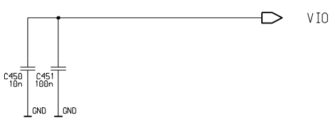
Decoupling capacitors for 1st flash
