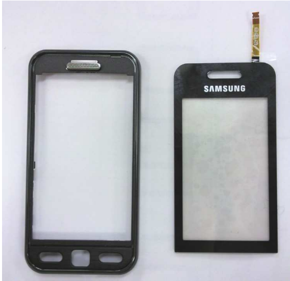
Disassembled FRONT and TSP.
