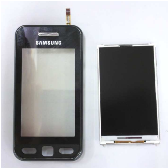
Disassembled FRONT and LCD.
