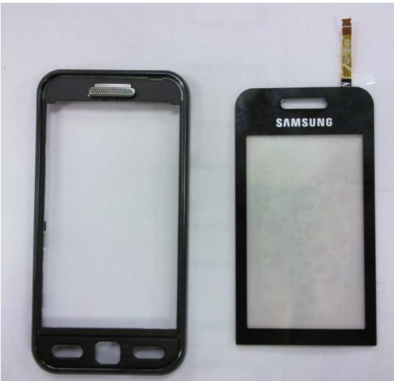
Disassembled FRONT and TSP.
