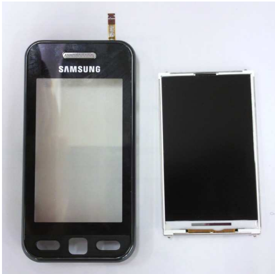
Disassembled FRONT and LCD.
