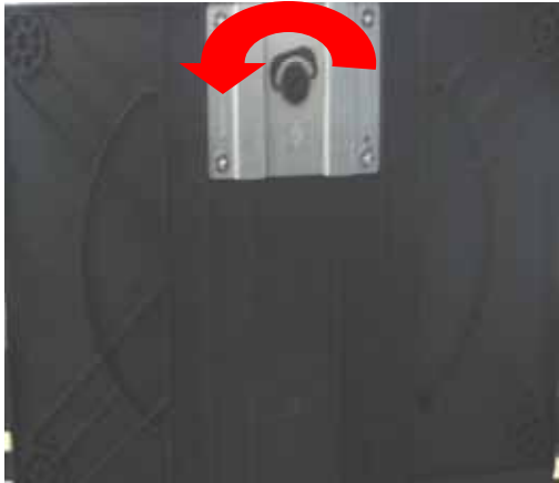
Remove the base ass'y. Turn the screw by using the screw handle.
