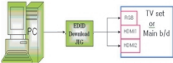
(Fig. 2) Connection Diagram of DDC download
