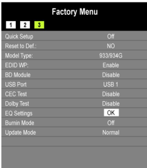
5. Select the appropriate model type by Right/Left Arrow key on the Remote. Model type is written on the rating label.
