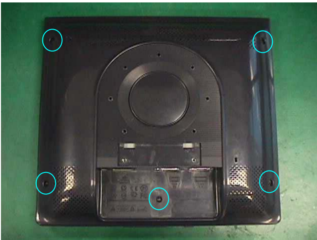
R. Assembly the Upcase (5 screws) and the Base (2 screws).
