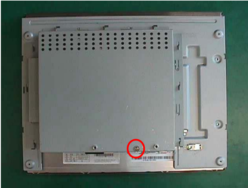
M. Assembly the Main Cover with the Main Bracket. (1 screw)
