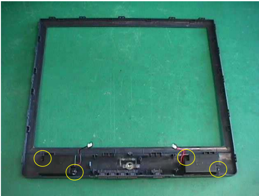
A. Screw up Speaker Drivers on the Bazel. (4 screws)
