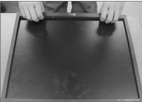
1. Pull the front cover upward. 2. Then, let the all latches are separated. 3. Put the front face down.
