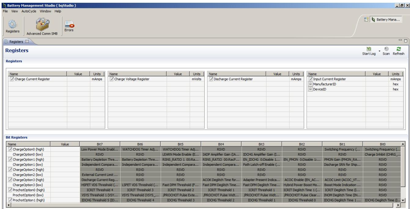
Figure 3. Main Window of bq24780S Evaluation Software
