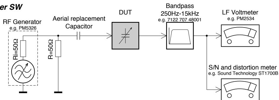
To avoid atmospheric interference all AM-measurements have to be carried out in a Faraday«s cage.
