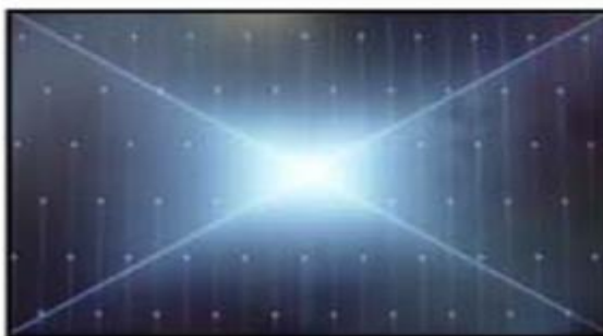
Solder defect, Short/Crack
