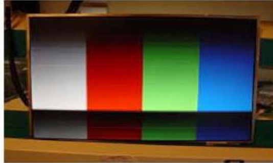
Horizontal Block Gate TAB IC Defect
