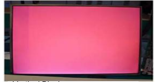
Vertical Block Source TAB IC Defect
