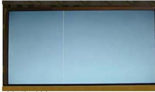
Vertical Line Source TAB IC Defect
