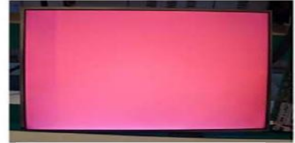
Vertical Block Source TAB IC Defect
