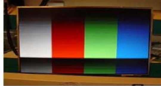
Horizontal Block Gate TAB IC Defect
